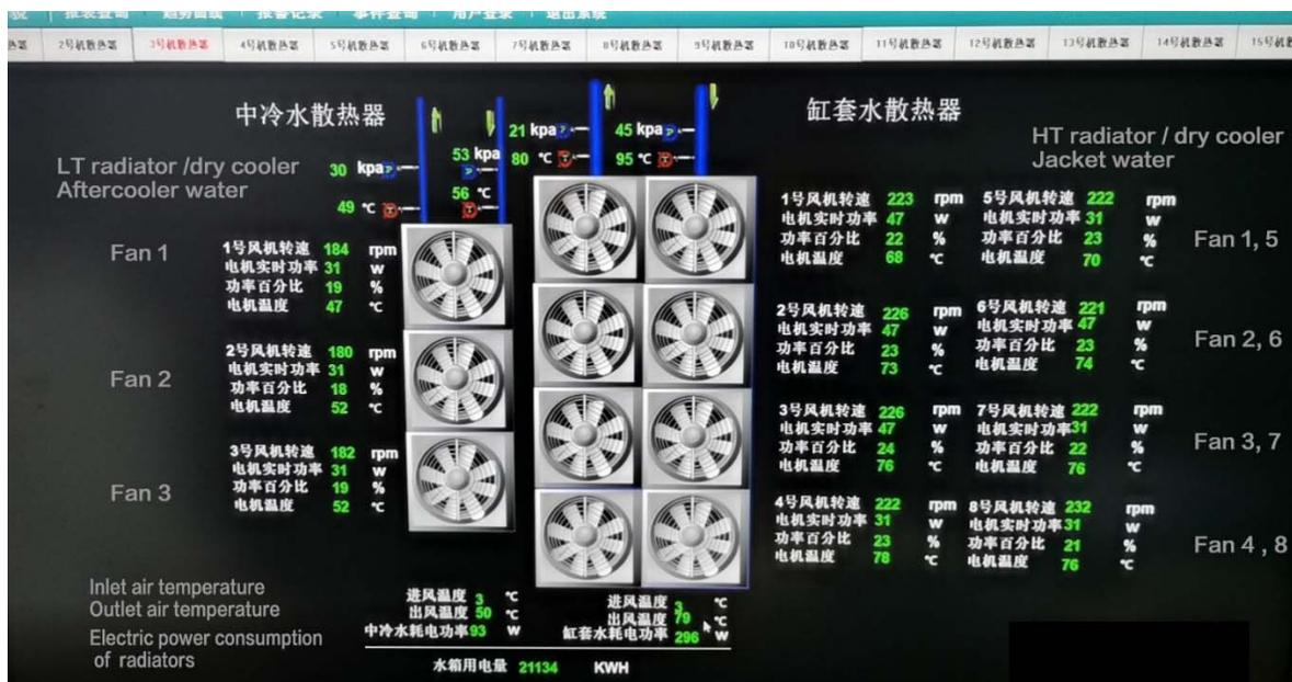
Figure 4. Real time monitoring of operational status of new radiators in Qinshui Jinmei
